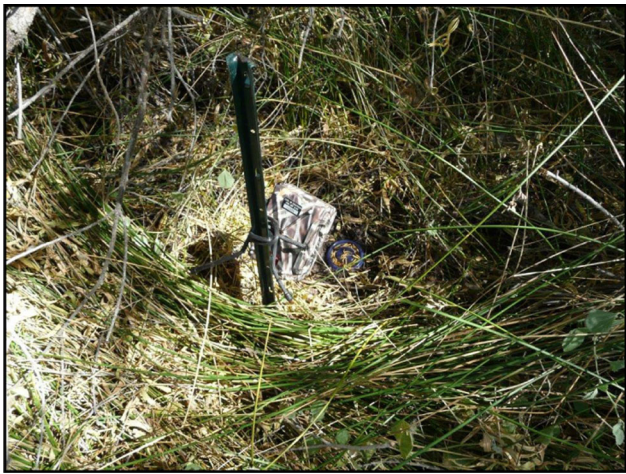
Figure 2. Example setup of a Reconyx close-focus automated camera station to detect Buena Vista Lake shrew ( Sorex ornatus relictus ) at Wind Wolves Preserve, Kern County, California, USA, in October 2016. The camera was attached approximately 20 cm off the ground to a 0.5-m metal t-post. To attract S. o. relictus , a small plastic container (approx. 9-cm diameter, approx. 7 cm deep) filled with polyester fiber batting and approximately 10 live mealworms was buried and pinned to the ground with a 15-cm nail. We placed approximately 30 dried mealworms on top of the container. Bait stations were positioned approximately 50 cm in front of each camera.
